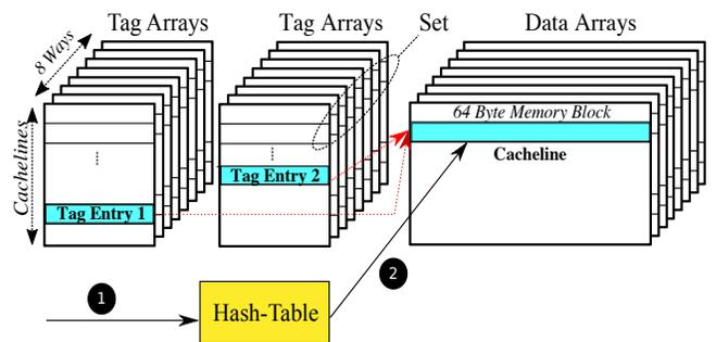
**Figure 4.** Last-Level Cache (LLC) implementing Deduplication (Dedup). Dedup enables multiple tags to point to the same cacheline containing a common memory block. During the LLC insertion of the memory block, Dedup uses a hash-table of the most recently used data values to identify exactly identical cachelines.
