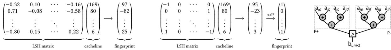
**Figure 6.** Left: computing the fingerprint of a cacheline using dimensionality reduction. Centre: a hardware-friendly variant developed for Thesaurus. Right: Hardware implementation using an adder tree and a comparator.
