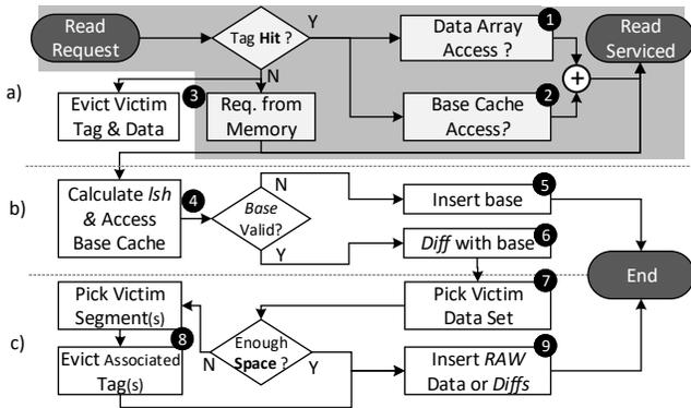
**Figure 12.** Processing a read request in Thesaurus: (a) critical-path lookup sequence; (b) cluster ID computation for new data brought in by a miss; (c) insertion of new data and possible data array evictions. Shaded steps are on the critical path, while unshaded steps are performed in parallel with servicing the read request.
