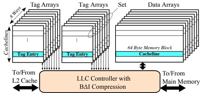
**Figure 3.** Last-Level Cache (LLC) implementing BAI Compression. The LLC has multiple tags per cacheline to store additional tags for each of the compressed memory block within the physical cacheline.
